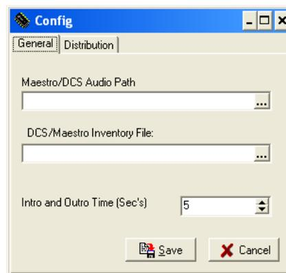
First, set the **Maestro/DCS Audio Path**. This designates where DCS or Maestro audio files you wish to play are located. This can be a UNC path or a standard path. Use the ellipse button adjacent to the field to pop up a folder selection dialog. The audio path is the only setting that is **required** – XPlay has to know where to find audio files to play!
